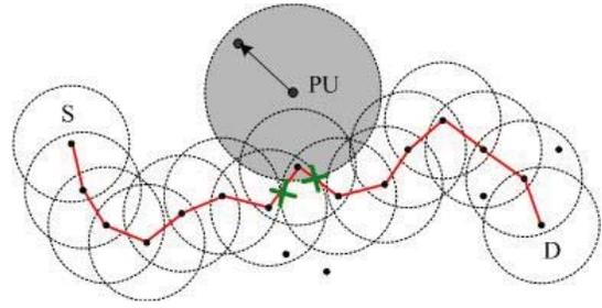
Fig. 1. Impact of frequency diversity on network connectivity
