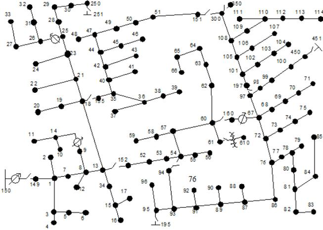
Fig. 3. The IEEE 123-bus test system
