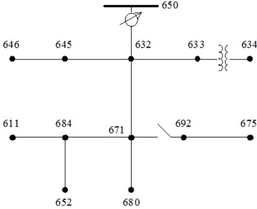
Fig. 2. The IEEE 13-bus test system
