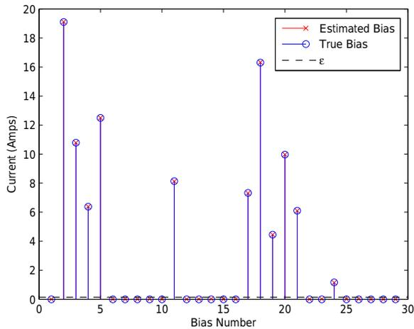
Fig. 4. Energy theft detection in the 13-bus system.
