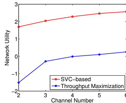
Fig. 2. Performance comparison of the proposed SVC-based scheme and Throughput maximization scheme. Radio number is 2, Channel number changes from 2 to 6.
