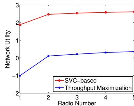
Fig. 3. Performance comparison of the proposed SVC-based scheme and Throughput maximization scheme. Channel number is 5, Radio number changes from 1 to 5.
