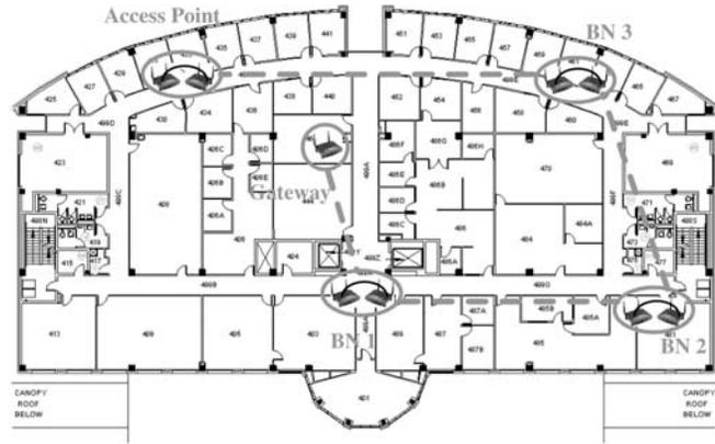
Fig. 5. WMN testbed placement (fourth floor in the New Engineering Building, University of Florida).
